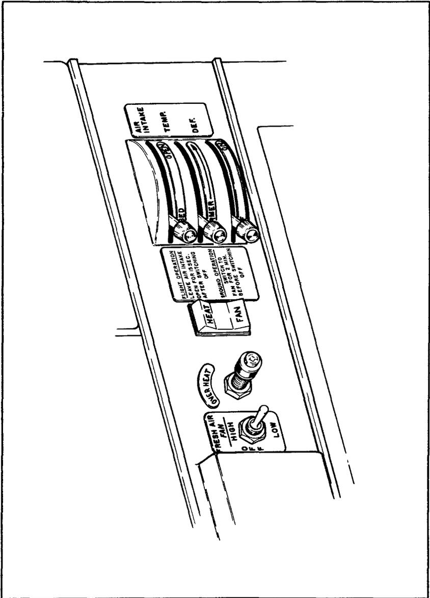
HEATING, VENTILATING & DEFROSTING CONTROL CONSOLE
